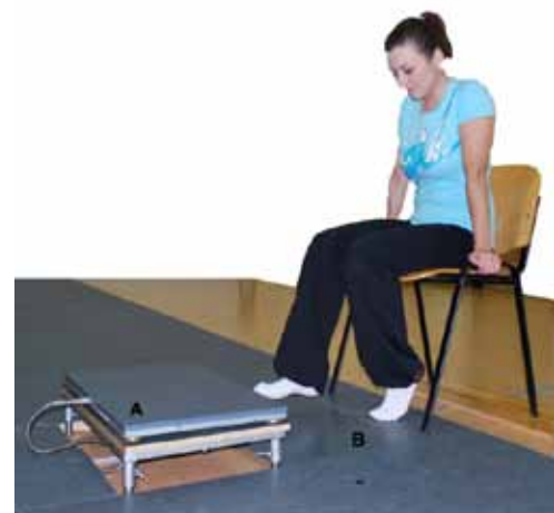
Figure 2. The experimental setup. Rhythm reproduction with the lower limb on a Kistler force plate (B)
